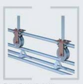
Flange/Guide roller 30 kN, Steel wheel Ø 200 mm Installation height 300 mm
