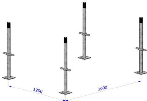
1 Set out according to the design drawing the Baseplates or Basejacks and set the Nut to the required height (not more than 500mm spindled out).
