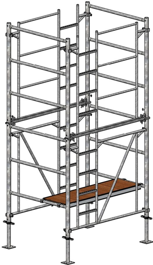
6 The next Frames can be mounted by sliding the snap-lock in the slotted hole of the top bracket and the frames verticals on the connector. The snap-locks at the top and the lock pins at the bottom will secure the Frames.
