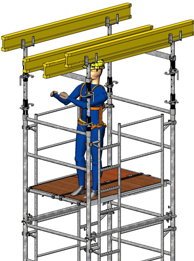
9 The finished support tower. Workmen can bring the beams, standing safe on the top platform, to the correct height.
