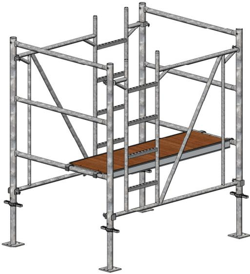
4 A Platform or Platform with lid may be mounted to ease erecting the next frames.
