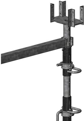
The secondary adaptor can be adjusted independent from the standard adaptor, to be able to support two different levels. Particularly interesting when a concrete slab with integrated beams have to be supported.
