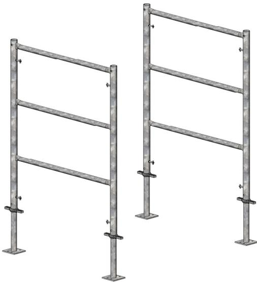
2 Mount two Frames 1.50m on the Basejacks. Check the level of both Frames and check whether the Frames are on the same height.
