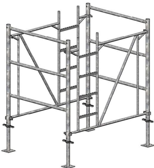
3 The Entranceframes can be mounted on the snap-locks of the Frames, by sliding the bottom bracket slotted hole over the bottom snap-lock and turning the top bracket over the top snap-lock. The tower will be stable now.
