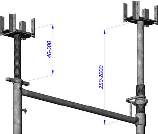
The adjustment of the top jack is also between 40 and 500mm. For the innertube the hole pattern will be the limitation factor. Note that the load capacity depends on the spindle height for jacks or extension height for innertubes.
