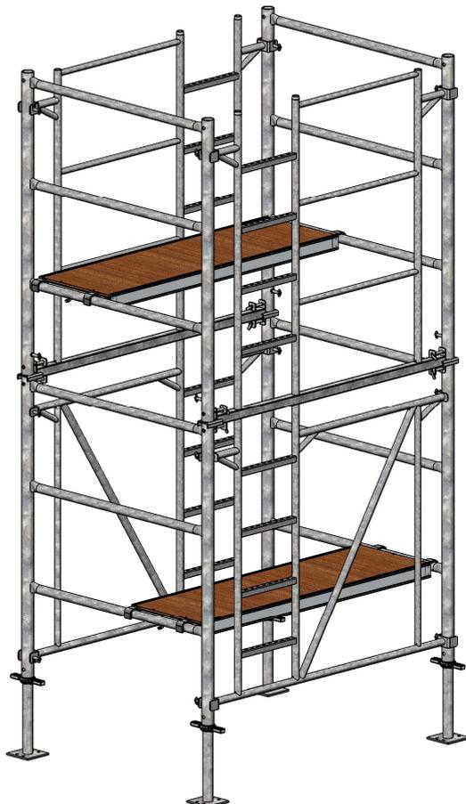
7 A Platform or Platform with lid is mounted to be able to build the next level.
