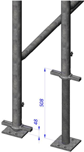
The adjustment of the base jack is between 40 and 660mm. However, it must be considered the maximum spindle distance between bottom plate and nut should be less than ca 500mm.
