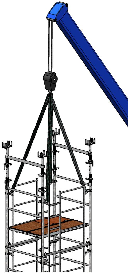
11 For hoisting and moving the tower four slings can be tied through the tubes forming the bracket support. The base jack can be secured with the Jack-lock.
